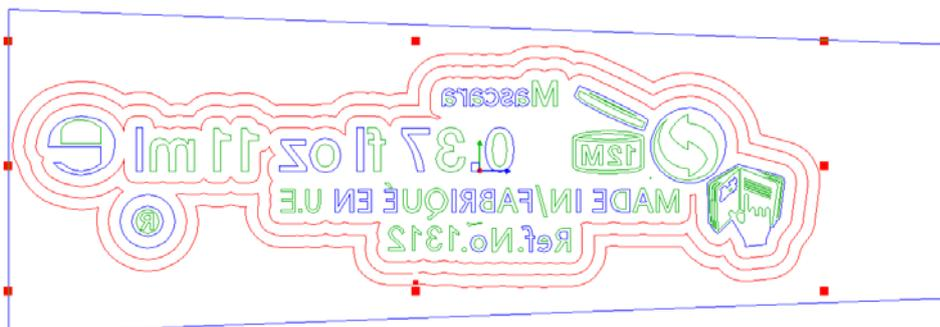
This multiple offset function allows several offsets to be linked together, one after the other. You can quantify the **Number** and size of the **Offset** depending on the tool. All angle management options remain possible (radial, right angle or chamfered).
