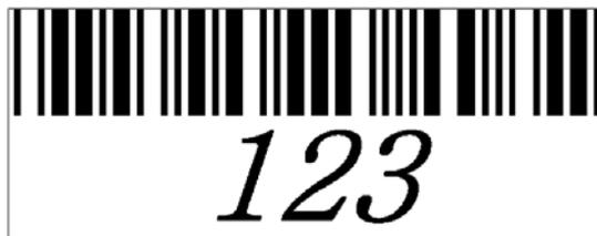
With a **Bar width** = 0.5 mm, a total width = 36.75 mm is obtained.
